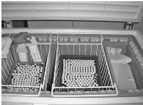
Fig. 2: Vaccine storage in ice-lined refrigerator.
